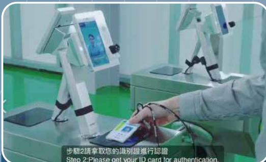
The system uses AI image processing technology for real-time body temperature measurement. It automatically sounds an alarm if it detects an individual who is not wearing a face mask. The system improves the efficiency and quality of overall disease prevention measures and can be used to improve its performance with the big data from measurement results.
