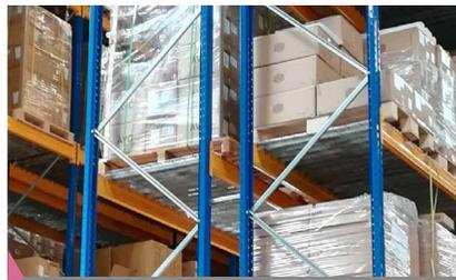
Czech Plant - Installation of side railings of shelves to stop products from falling
