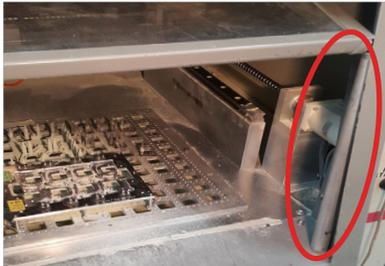
● Hsinchu plant—Safety control rod next to the router machine
