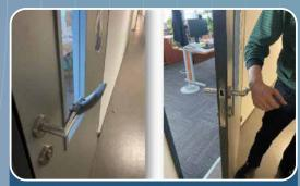
Employees used the 3D printer in the plant to design an innovative "door opener" so that users can use their arm or elbow to open doors without touching the door handle. This measure significantly reduces the possibility of spreading the virus with door handles.
