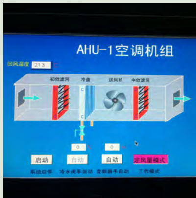
Variable-frequency control of Air-conditioner.
