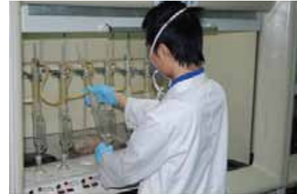
Extract Polybrominated Biphenyls and Polybrominated Diphenyl Ethers Through a Soxhlet Extractor
