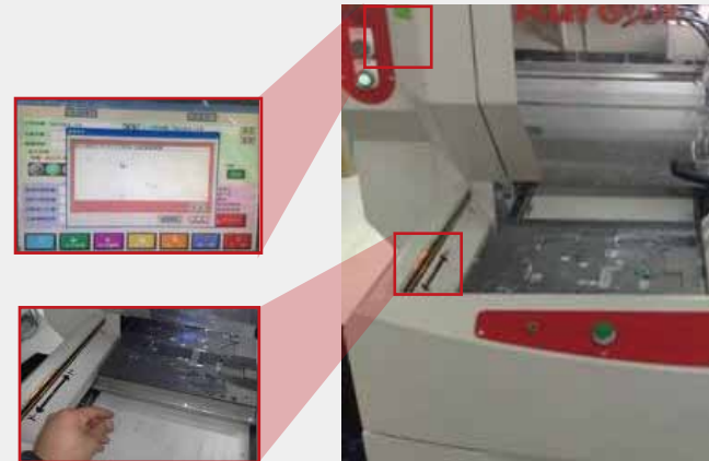
For machines with moving parts that cannot be covered, an infrared sensor is installed for protection.
